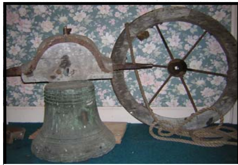
The Bell with its "Napoleon's Hat", rocker and bell rope before it went on loan to Anstruther fisheries Museum, which was before it was sand-blast cleaned by Classic Cars Alyth and restored to its present condition.
